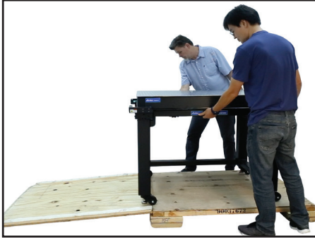
The roll-off packaging simplifies table rigging
